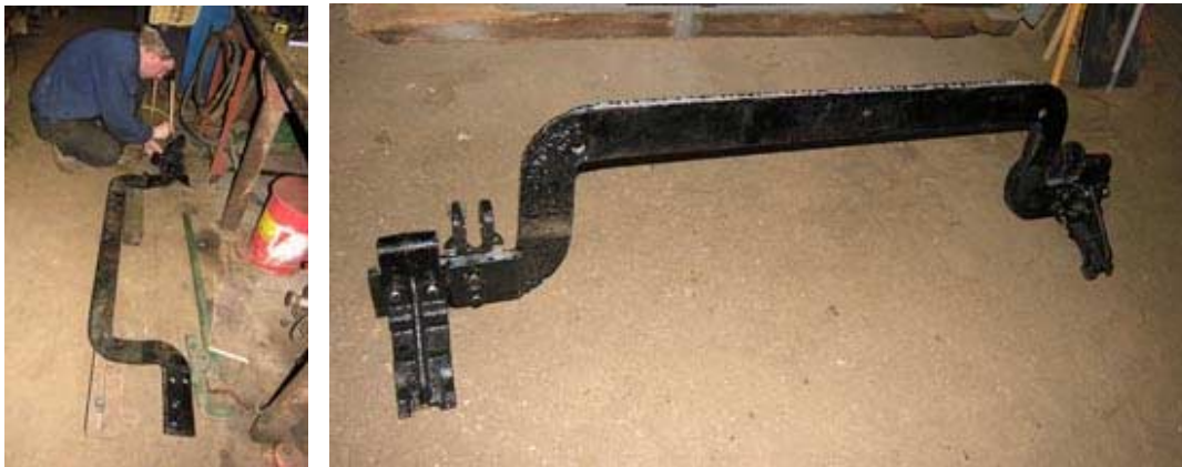
Bill Pollman installing brake shoe head on rebuilt brake beam
