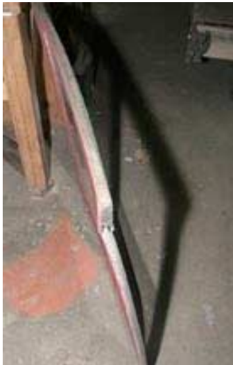
Bent cab sash
