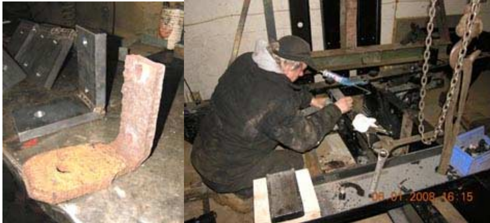
Old and new motor mount angles (before trimming corners) Bill Pollman installing them on the truck frame
