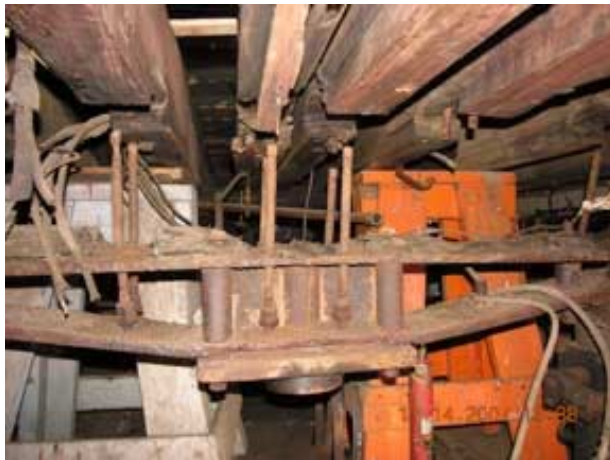
No. 2 end original bolster and Donald Curry installing new one
