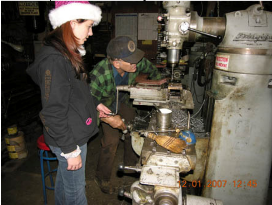
One of Santa's Elves (Chelsey Pino) watching Dean Look prepare to machine a new end for a brake beam
