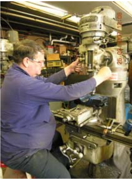
Chuck milling out dowel pins
