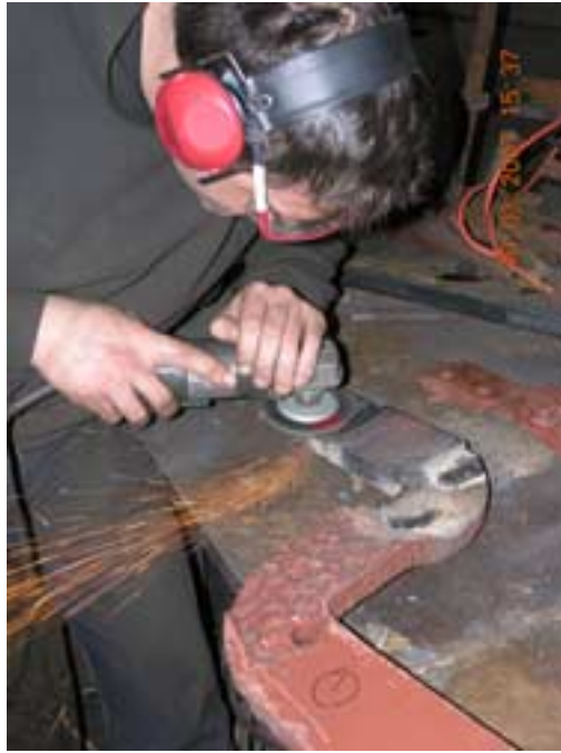
Randy Bogucki grinding the new brake beam end. Note the extent of the pitting.
