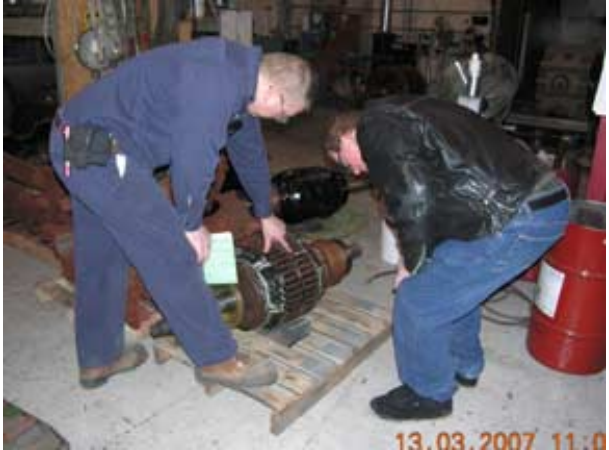
Roger Paradie and Dan Cohen inspecting the questionable motor armature.
