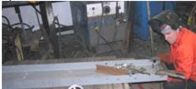
Bill Pollman welding extension 'ears' on truck transom.
