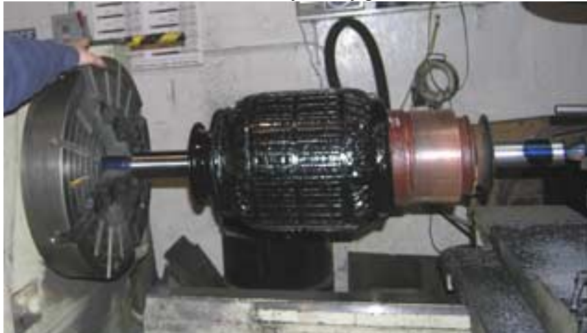
Armature in the lathe for truing the shaft. (The blue area on the right shaft is a 'low' area.)
