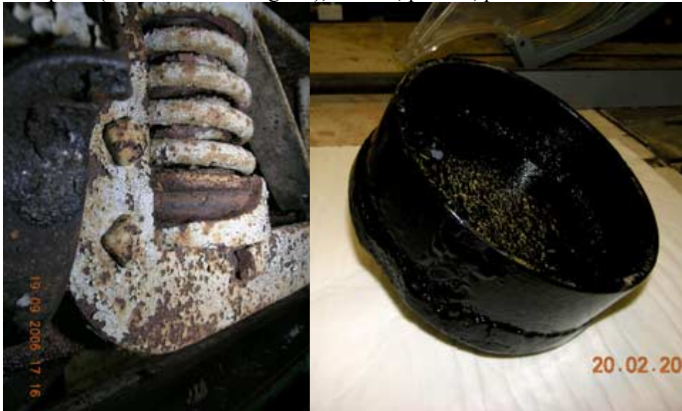
Original cracked spring cup and rebuilt and repainted 2 one.
