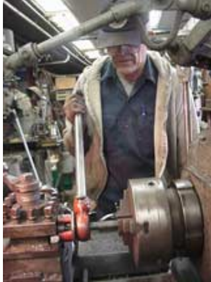
Dean Look threading a rod before installing bolt-head
