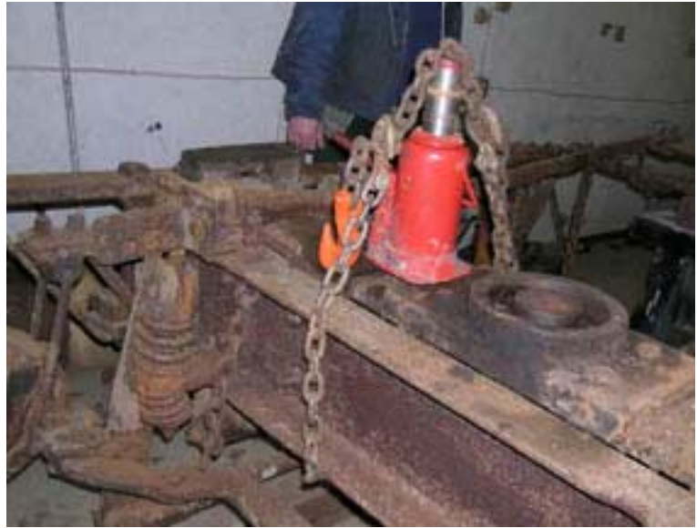
Randy Bogucki driving out swing link bracket bolt Squeezing the bolster elliptic springs
