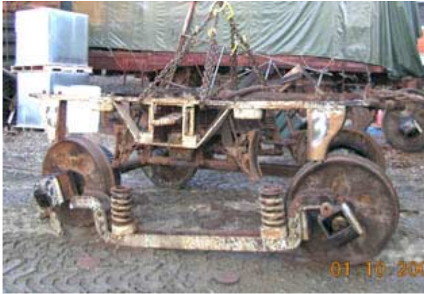
Lifting the truck frame
