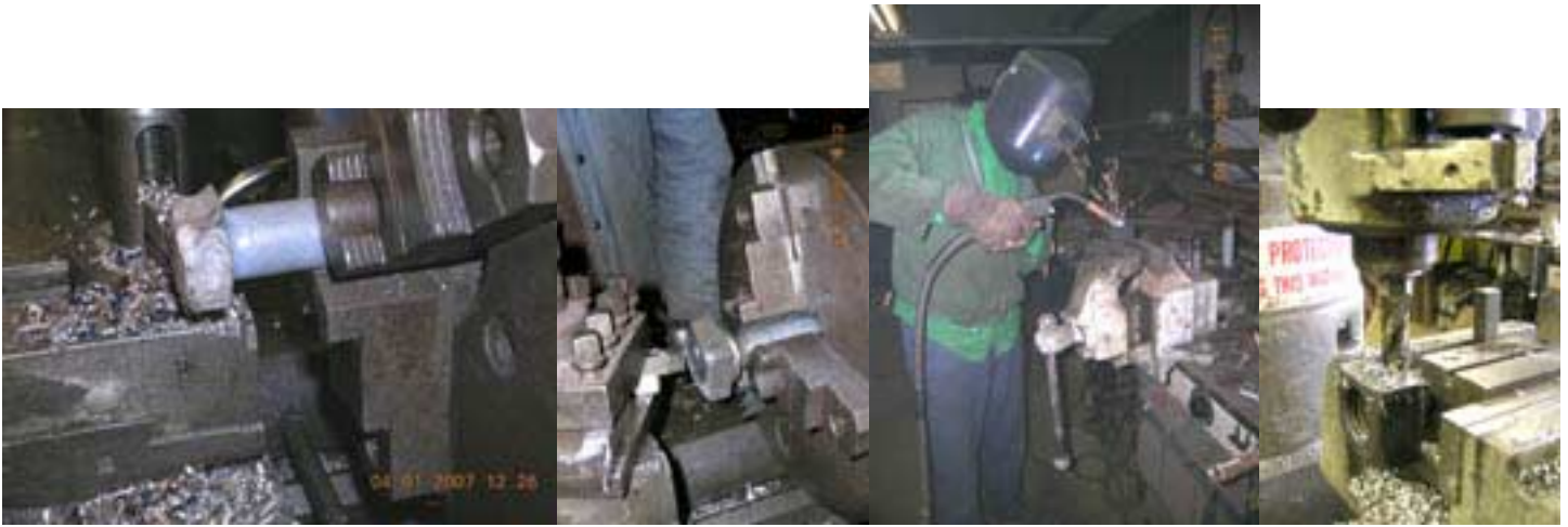
Remaking the square-headed motor frame bolts Dean Look welding
