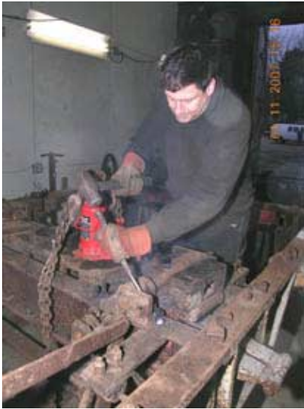
Randy Bogucki driving out swing link bracket bolt Squeezing the bolster elliptic springs
